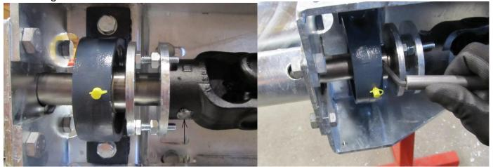
Release the cutter on the pump housing.
