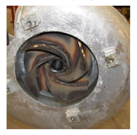
Pull out the drive shaft and the impeller together. If there is runout in the drive shaft, push out the breaker bolt which attaches the impeller to the drive shaft.
