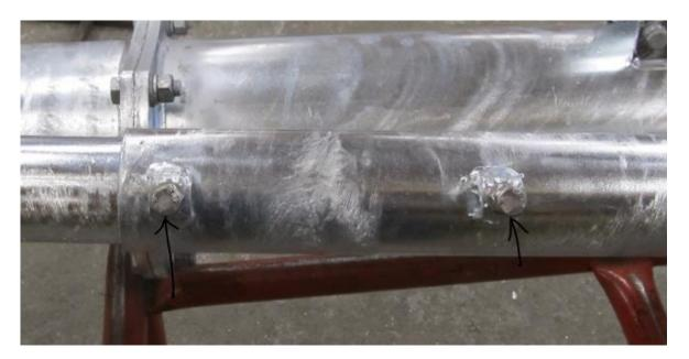
Release the cover tube where it is attached to the pump housing.
