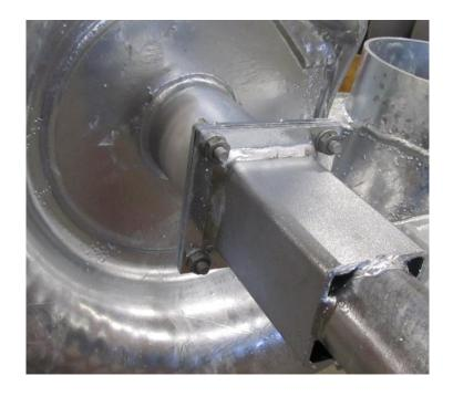
Push out the breaker bolt which secures the drive shaft to the double joint. Release the set screws on the bearing.
