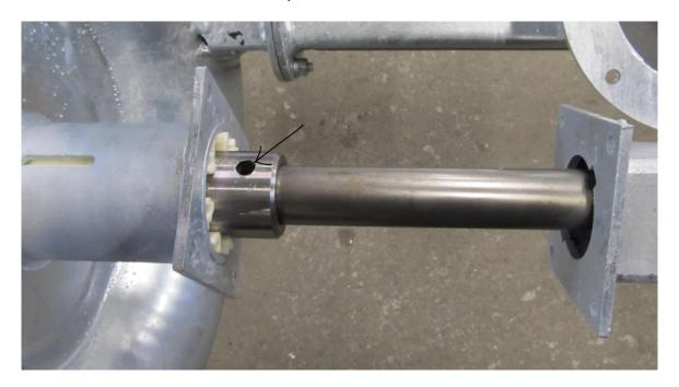
Remove the impeller from the drive shaft.
